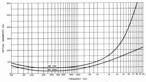
fig. 1. Critical bandwidth of the human ear as a function of frequency.
